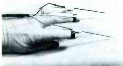
Fig. 3 The three finger probes have sharp tips, making it easy to penetrate insulation or corrosion, and allowing solid contacts with points on the circuits boards. One-hand operation frees the other hand to operate the switches of the tester.
