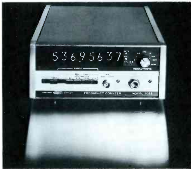
One example of a direct-reading frequency counter. Courtesy of Syton-Donner Corporation
