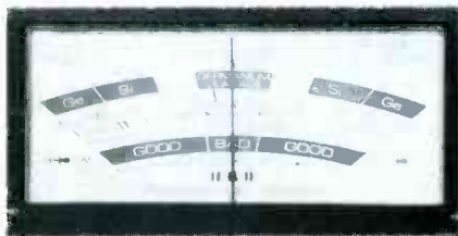
Fig. 2 This closeup of the meter face shows the areas that indicate silicon or germanium material, PNP or NPN polarity, germanium leakage, relative gain, and in-circuit good/bad scale.
