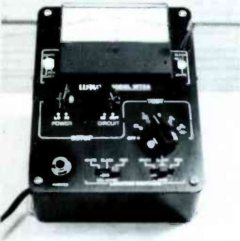
Fig. 1 The Wayne WT2A transistor tester is shown with a small transistor plugged into one socket, and with the switches adjusted for locating the base.
