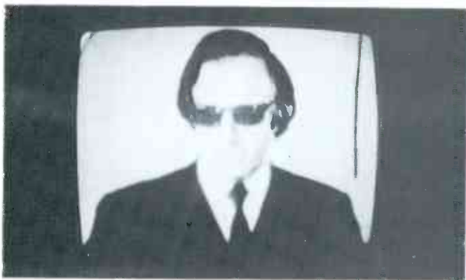
Fig. 1 Picture on the Zenith was nearly normal, except the focus was not sharp, and the size changed with brightness.
